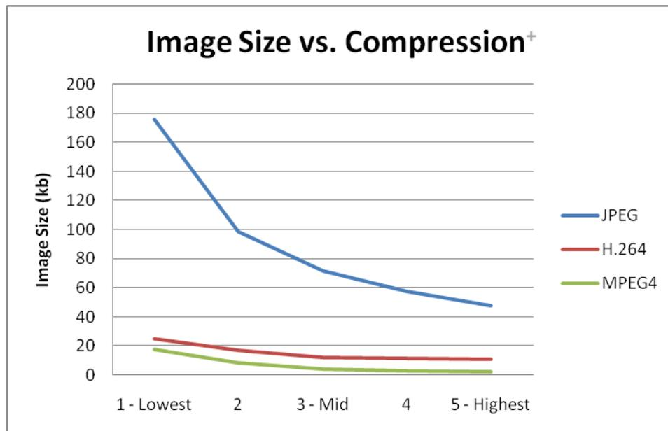
+ Image size data was averaged from the four cameras listed below. Only the Sony cameras support MPEG4. In the charts below, 'Dynamic Range' refers to the ratio of compression from maximum quality to minimum, and 'MJPEG:H.264' is a compression ratio based on image sizes at highest and lowest quality.
